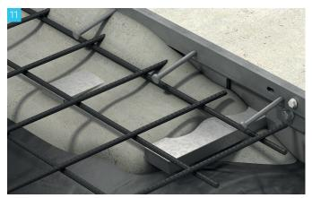
Place the specified slab reinforcement and pour concrete for the new slab. Ensure proper vibration is conducted in the freshly poured concrete to allow for compaction and elimination of air pockets. Care should be taken to not disturb the profile or dowels with the vibrator.
