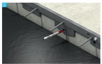
Align Isedio Dynamic Extend profile to the top edge of slab and mark drill hole points using a marker on the face of the slab through the pre-drilled holes in the profile.
